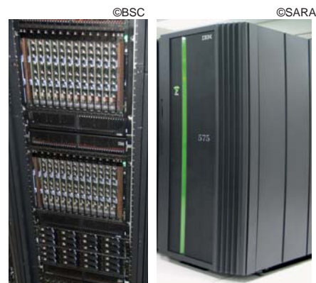
BSC in Barcelona will evaluate a hybrid prototypes combining IBM Cell and Power6 (picture in left) processors. SARA Computing and Networking Services (the Netherlands) will evaluate the IBM Power6 architecture (right).
